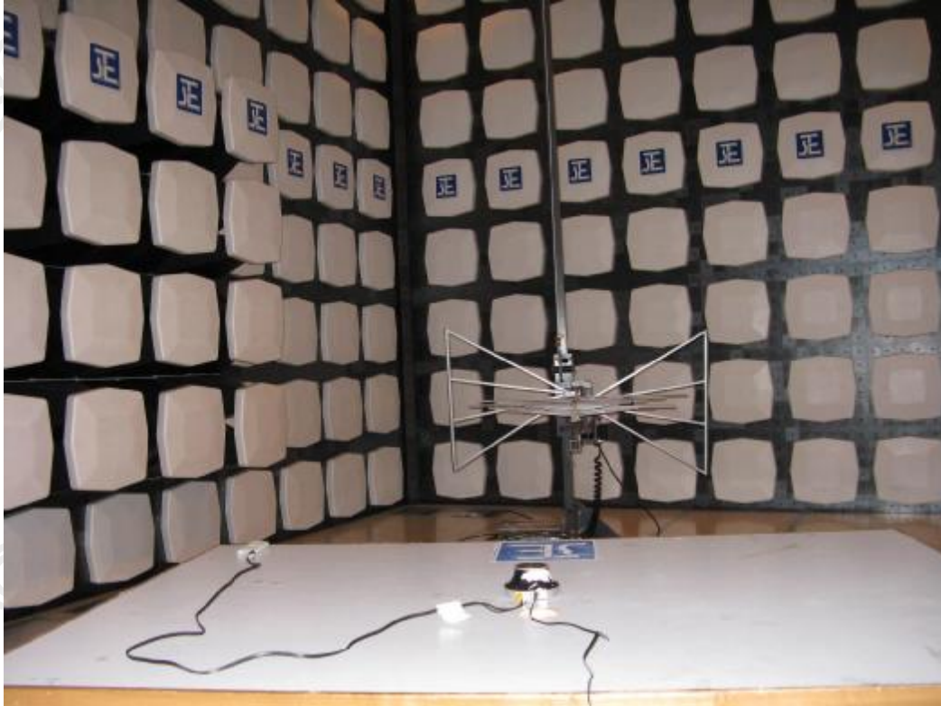
Measurement of Radiated Emission Test Set Up
