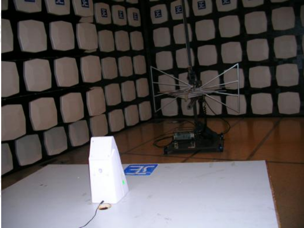
Measurement of Radiated Emission Test Set Up
