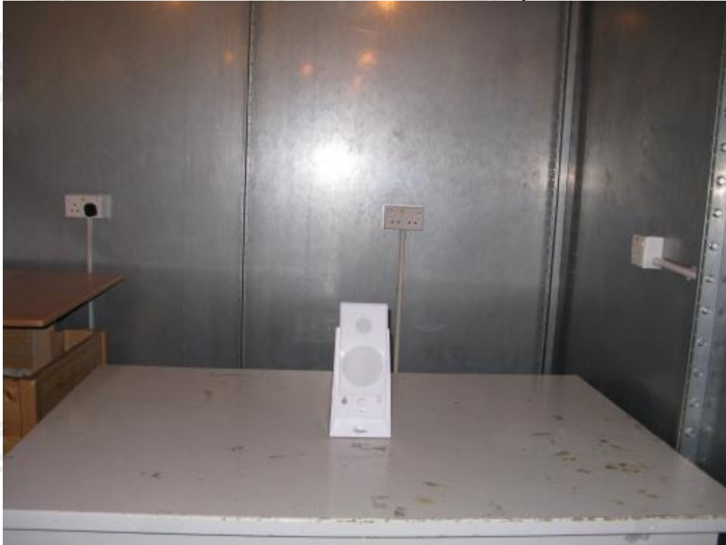
Measurement of Conducted Emission Test Set Up
