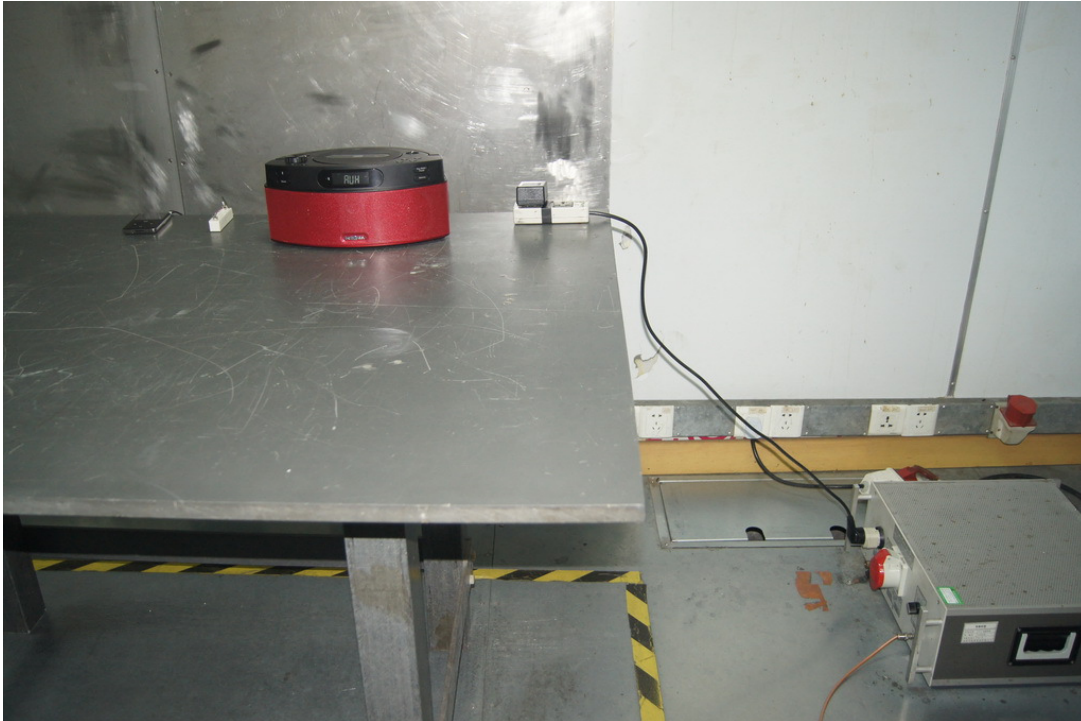
Photograph 6: Set-up for Radiated Emissions, below 1GHz
