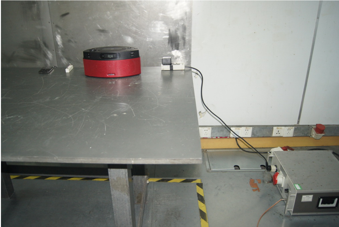
Photograph 6: Set-up for Radiated Emissions, below 1GHz
