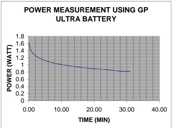
Even though the power droop is quite significant when measured using the different 3 types of battery, their power droop curve for battery + 6VDC is similar to that of using 6VDC only - See 1(b)(ii). As such, SAR measurement was carried out in the worst case configuration (Belt Clip Body Worn at Channel 4) after the EUT (using Energizer, Panasonic & GP Ultra Battery + 6VDC) has transmitted for 10 minutes. Shielding and ferrite dampeners are used on the wire of the external power supply.
