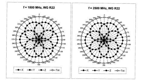
Isotropy Error ( $\phi$ ),  $\theta = 0^{\circ}$
