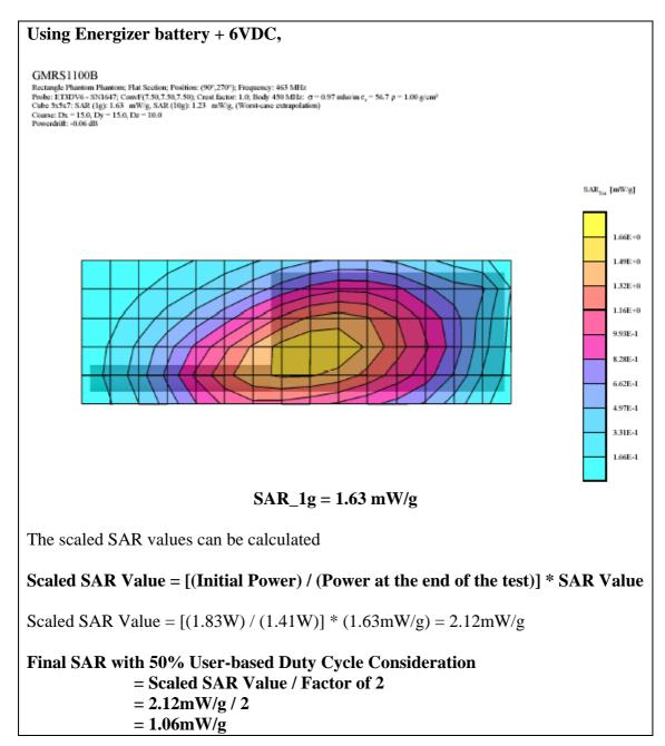
Alkaline AA non-rechargeable batteries are used for the SAR measurement. 3 brands commercial AA batteries are also investigated. They are Energizer, Panasonic and GP Ultra.
