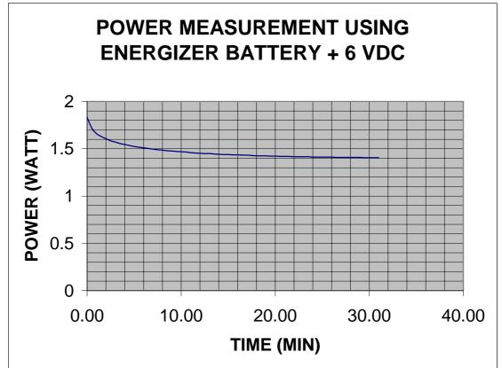
From the Power Vs Time Plot for Energizer Battery + 6VDC, it can be observed that the power droop after the first 10 minutes is less significant. That is the power is most stable after 10 minutes of continuous transmission.
