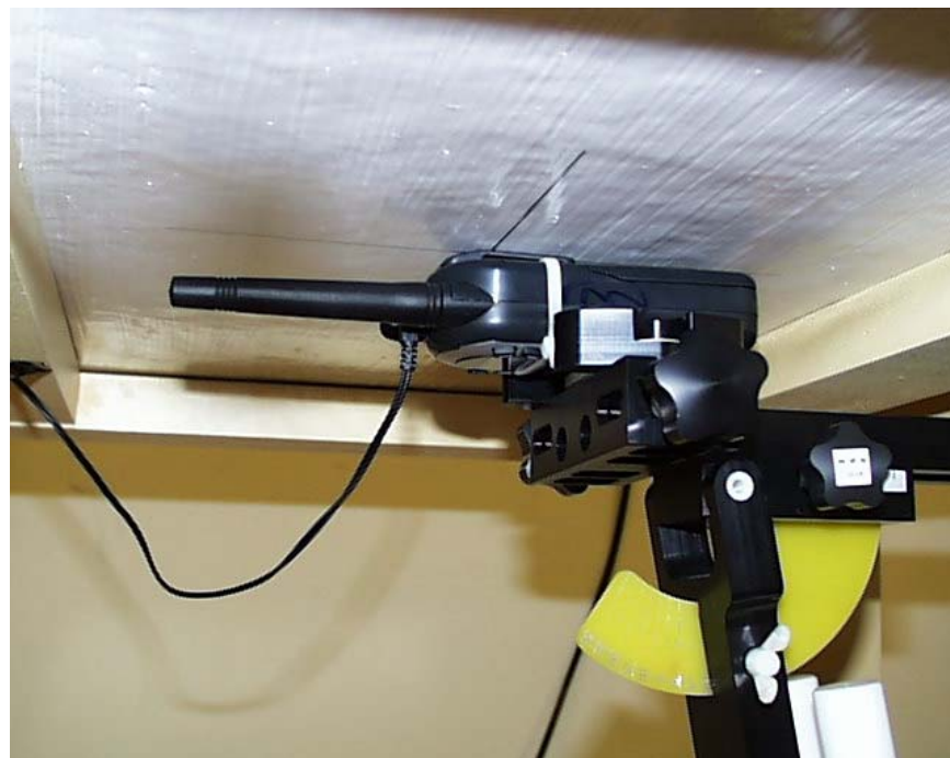
SAR Test Setup (Waist Position) – Closer View
