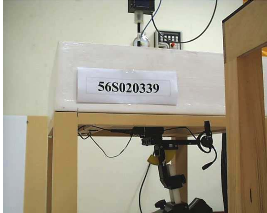
SAR Test Setup (Waist Position) – Far View
