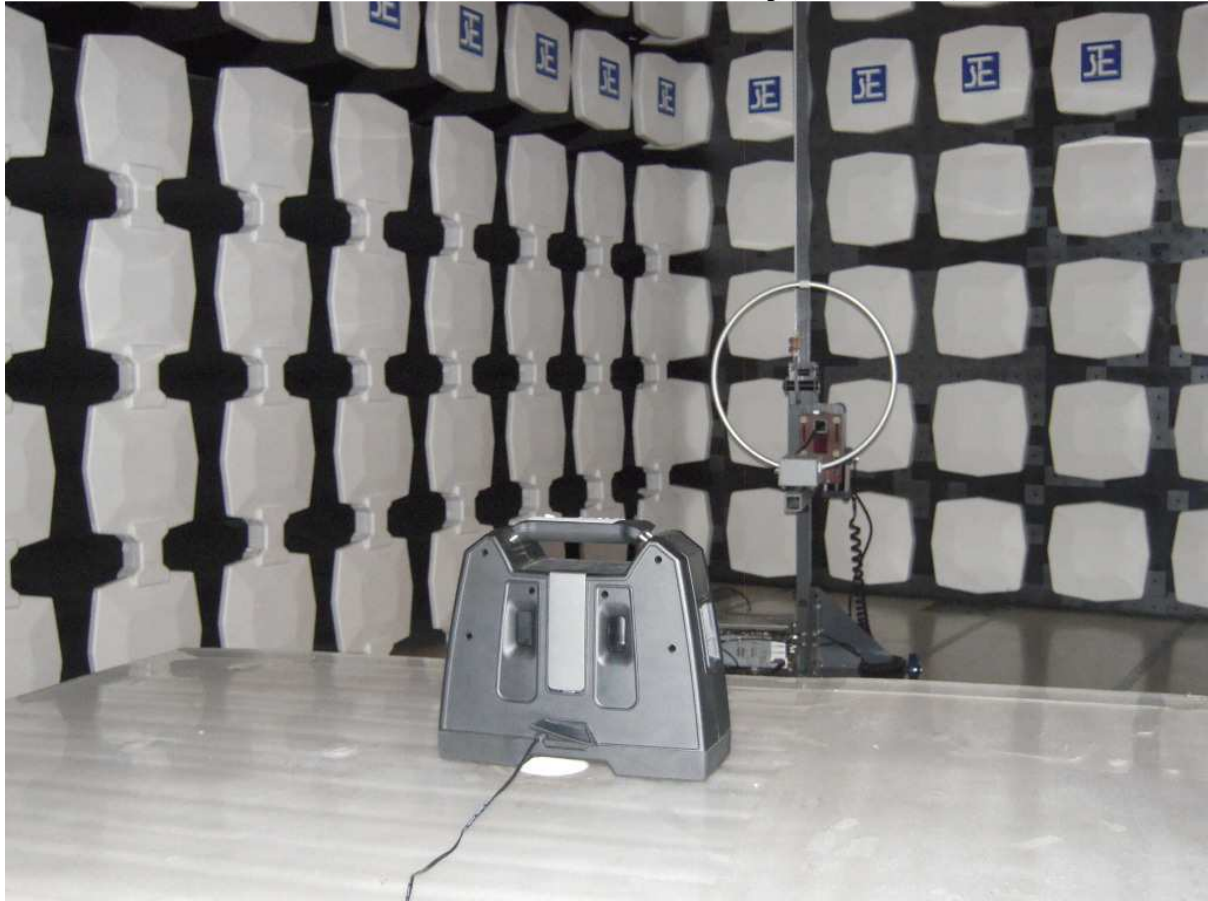
Measurement of Radiated Emission Test Set Up (Below 30MHz)
