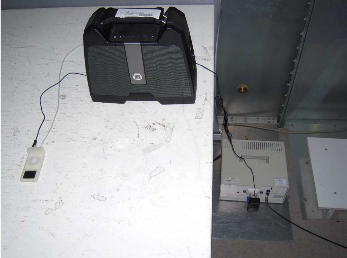
Measurement of Conducted Emission Test Set Up
