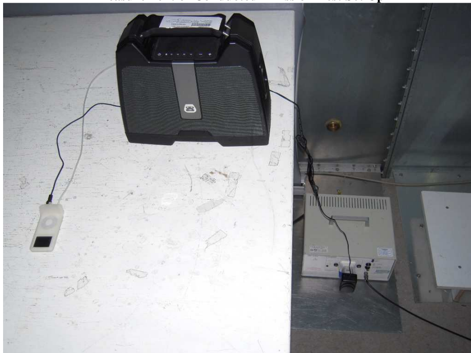
Measurement of Conducted Emission Test Set Up
