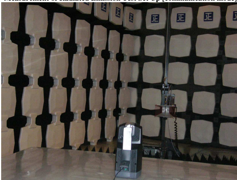
Measurement of Radiated Emission Test Set Up [communication mode]
