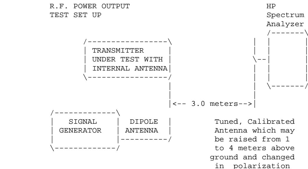
Equipment placed 1 meter above ground
