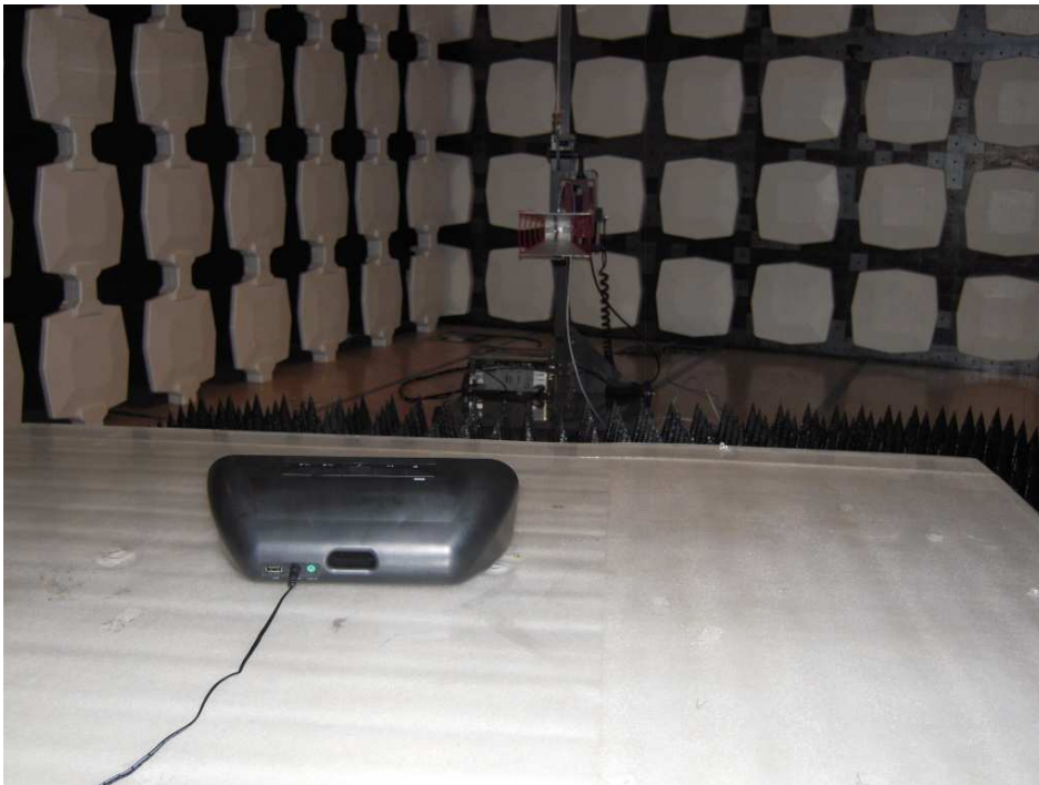
Measurement of Radiated Emission Test Set Up [communication mode]
