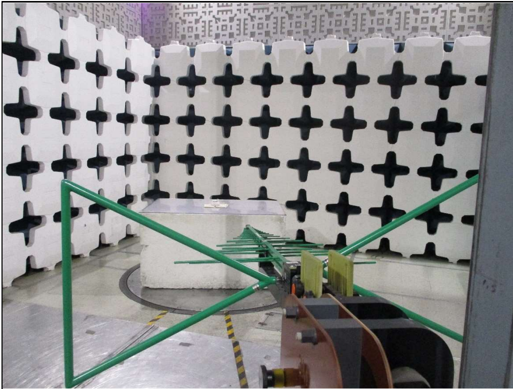
Test Setup for Spurious Radiated Emissions, 30-1000MHz – Antenna Polarization Horizontal
