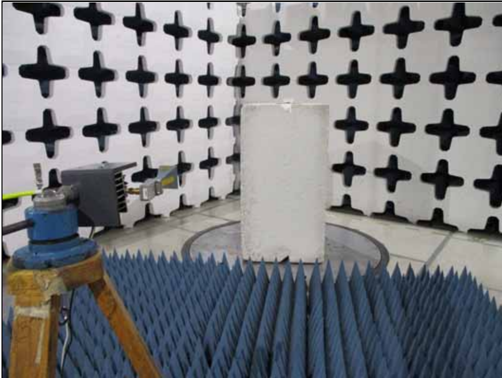
Test Setup for Spurious Radiated Emissions, 1GHz to 18GHz – Antenna Polarization Horizontal
