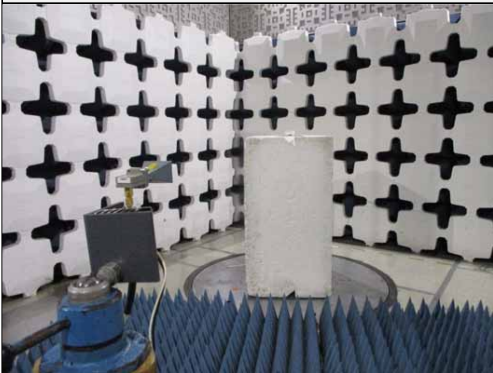
Test Setup for Spurious Radiated Emissions, 1GHz to 18GHz – Antenna Polarization Vertical
