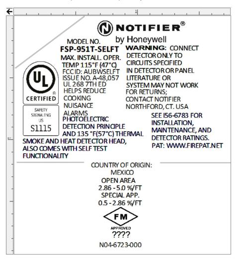
Photo/Heat Detector (FSP-951T-SELFT) Carton Label:
