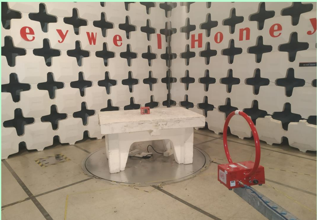
Radiated Emission Setup – 9 KHz to 30 MHz [ Perpendicular ]
