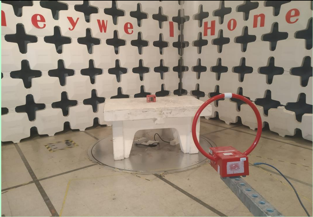
Radiated Emission Setup – 9 KHz to 30 MHz [ Parallel ]
