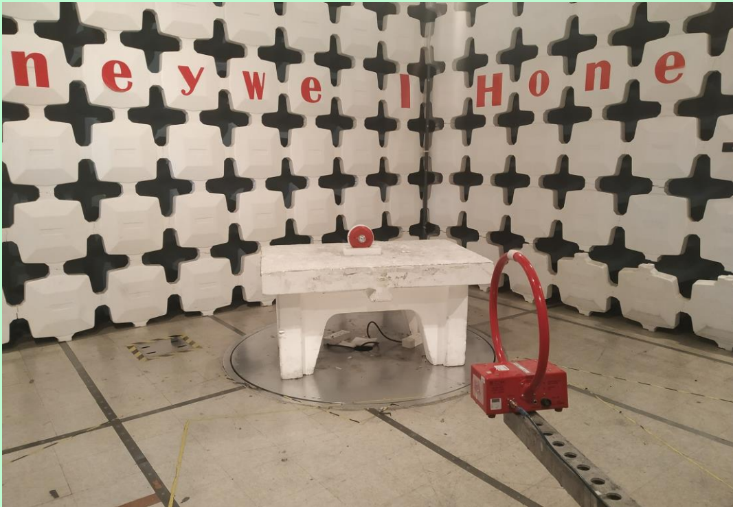
Radiated Emission Setup – 9 KHz to 30 MHz [ Perpendicular ]
