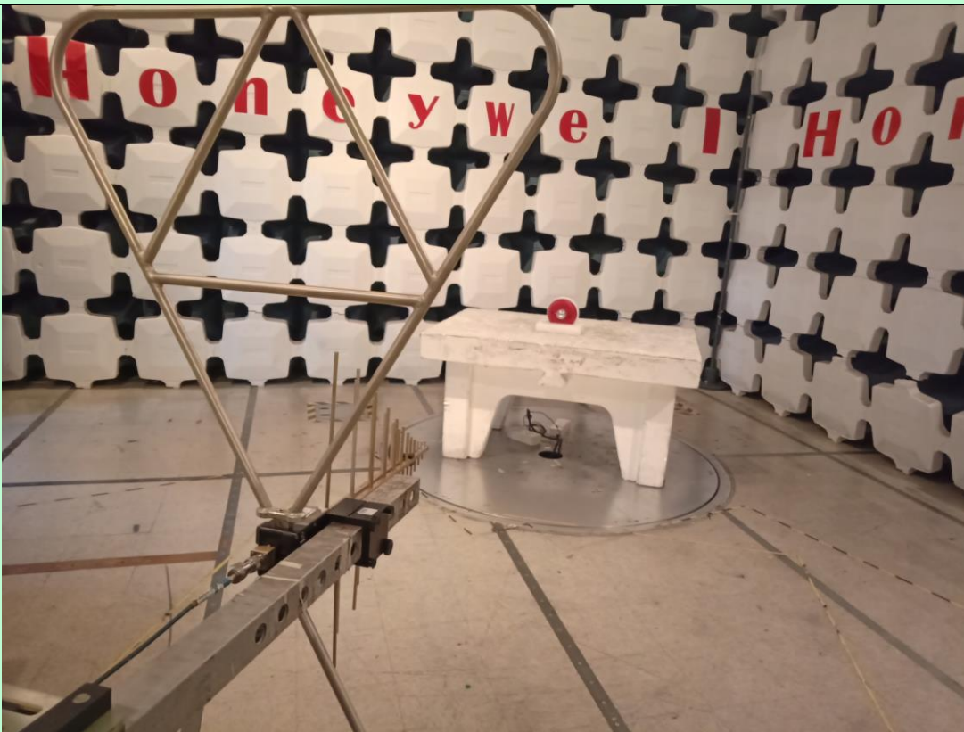
Radiated Emission Setup -30 MHz to 1 GHz [ Vertical Polarization]
