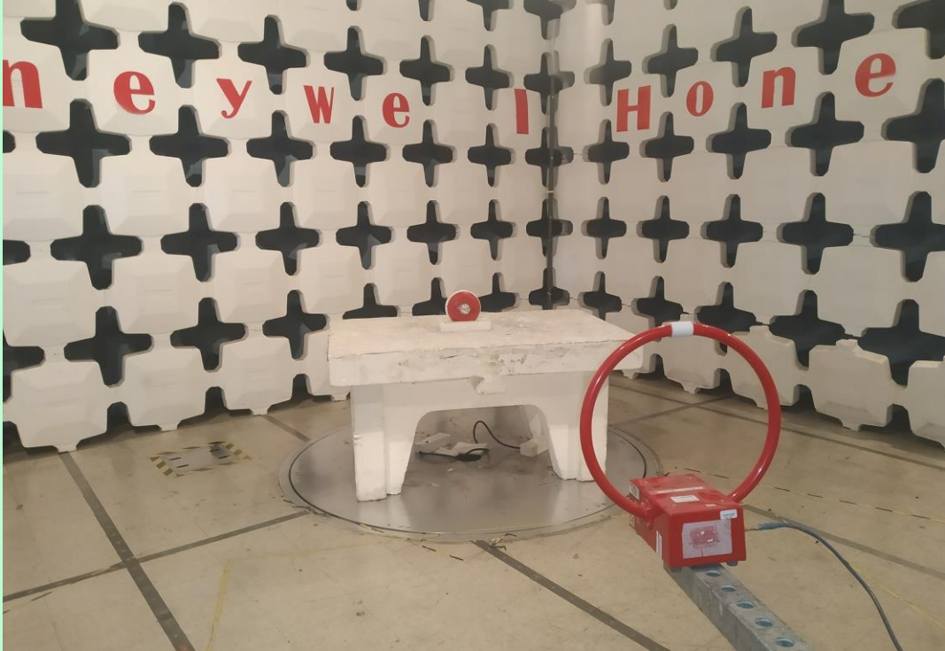
Radiated Emission Setup – 9 KHz to 30 MHz [ Parallel ]
