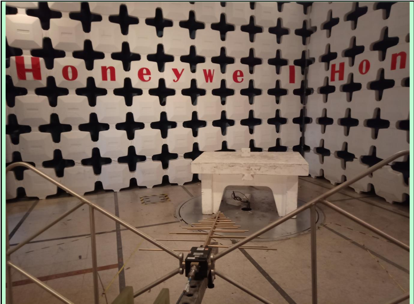
Radiated Emission Setup -30 MHz to 1 GHz [Horizontal polarization Polarization]
