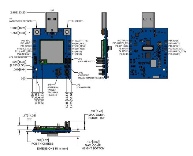
**Note:** The Reset and Wake buttons reset and wake the xDot processor.
