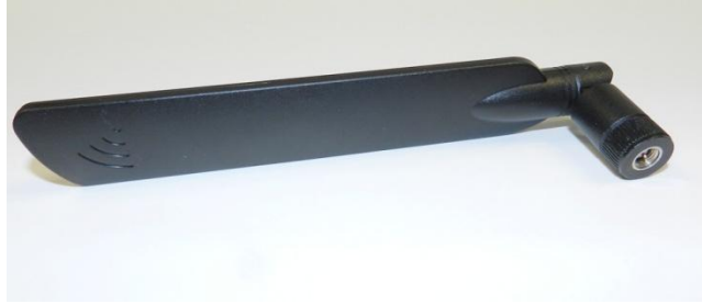
Figure (5) Laird Hepta-SM MAF94300, Cellular and Diversity
