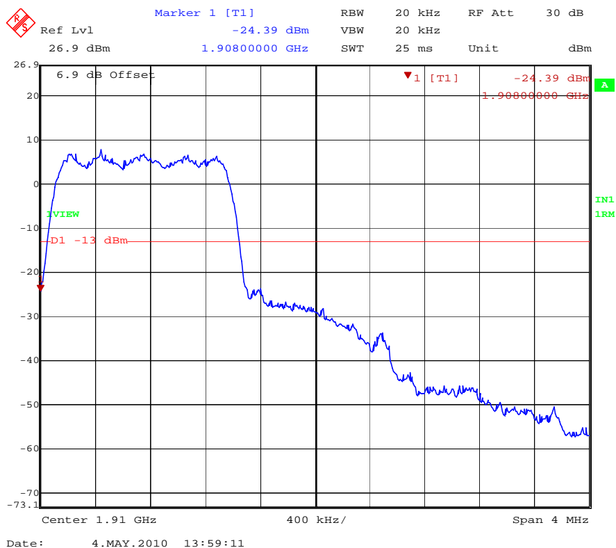
Figure 8-10: Emissions within 1 MHz of band edge, CDMA 1900 Channel 1175
