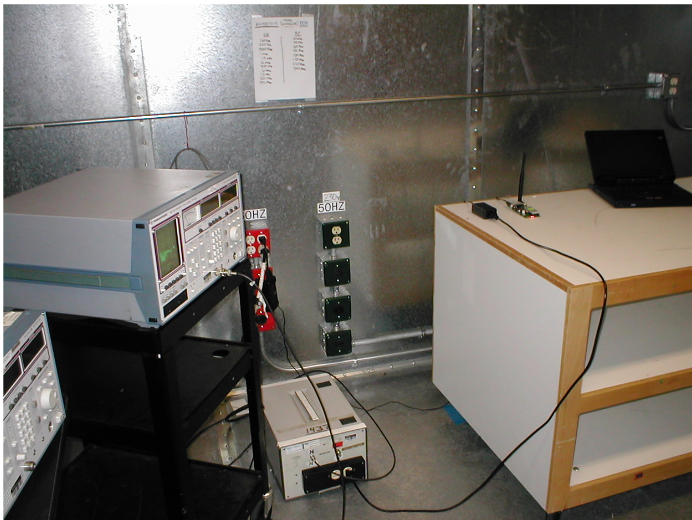
Test-setup photo(s): Conducted limits - AC power lines
