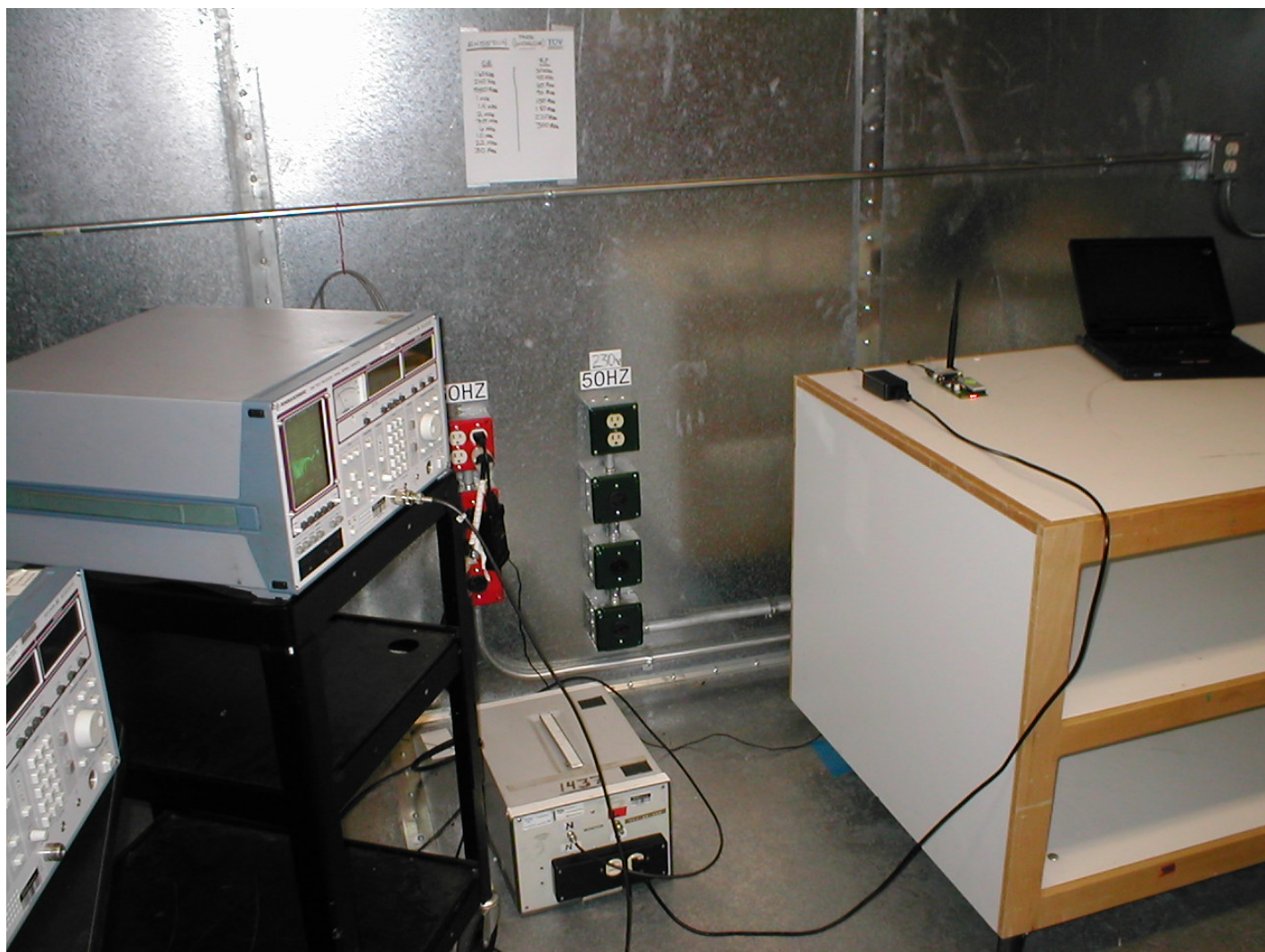
Test-setup photo(s): Conducted limits - AC power lines
