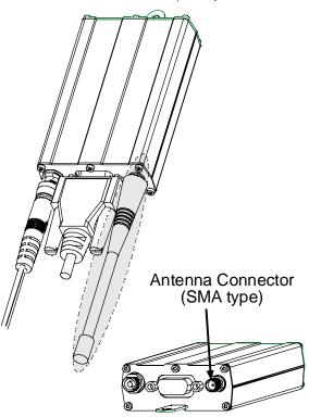
5. Connect both sides of the serial and control cable (15-pin Sub D connector on the modem side).
