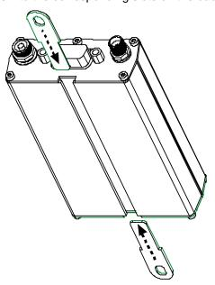
**NOTE**: Some MultiModem units will be shipped with a <u>single mounting bracket</u>. Slide it through the channel on the MultiModem chassis and secure with screws.
