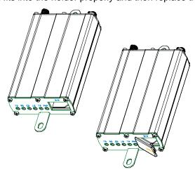
4. Connect a suitable antenna to the SMA connector (see specifications on page 5).
