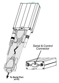
6. Plug the power supply cable into the modem.
