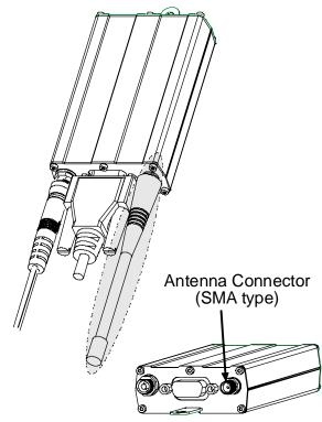
5. Connect both sides of the serial and control cable (15-pin Sub D connector on the modem side).
