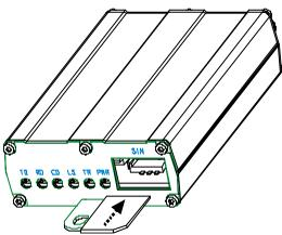
3. Verify that the SIM card fits into the holder properly and then replace the cover.
