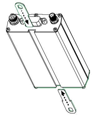
4. Attach the MultiModem with two screws to the mounting surface at the desired location on the equipment.
