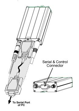
6. Plug the power supply cable into the wireless Multimodem.
