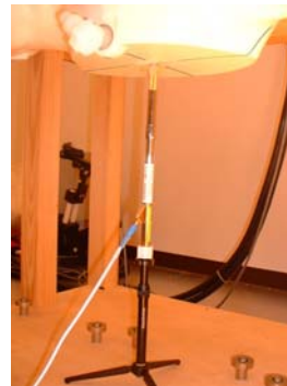
2450MHz System performance check setup
