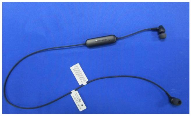
Bluetooth solution: WT200 Bluetooth version: V4.2 Bluetooth profiles: A2DP,AVRCP,HFP,HSP CODEC: SBC Speaker : 8mm (same as C7BT) Operation distance: 10 meter Battery: 80mAh VDL41030(400929) Charging time: about 1.5 hours Music playing time: 6.5 hours Phone call time: 6.5 hours Temperature : 5~40 °C
