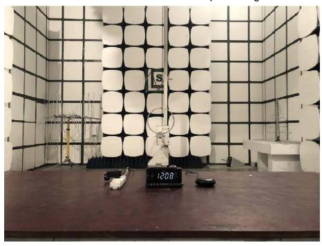
Radiated Emission below 1GHz-AC adapter charge mode
