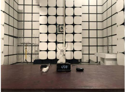
Radiated Emission below 30MHz-AC adapter charge mode
