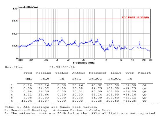
Remark: Measured at antenna position 0 degree and 90 degree, recorded worst case at 90 degree.
