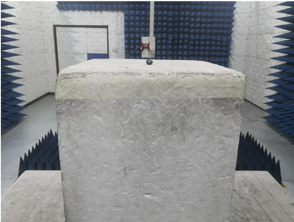
RADIATED EMISSION TEST SETUP ABOVE 1GHZ
