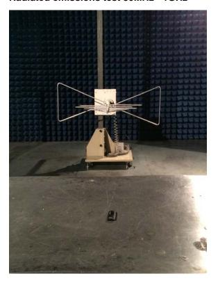
Radiated emissions test > 1GHz
