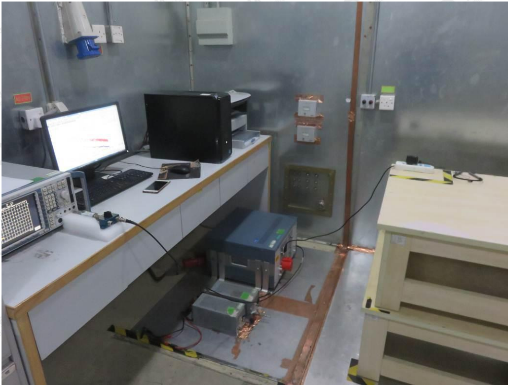
FCC RADIATED EMISSION TEST SETUP
