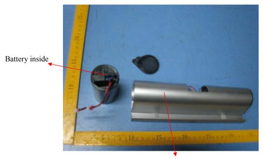
Remark: This battery and speaker box removed from left side of the device.
