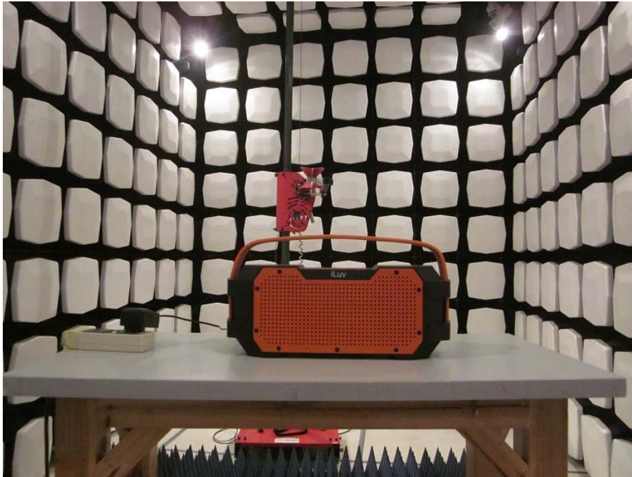
Measurement of Radiated Emission Test Set Up
