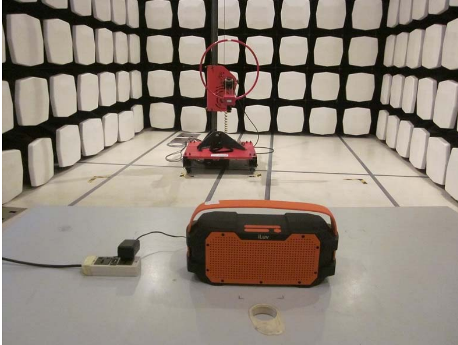
Measurement of Radiated Emission Test Set Up
