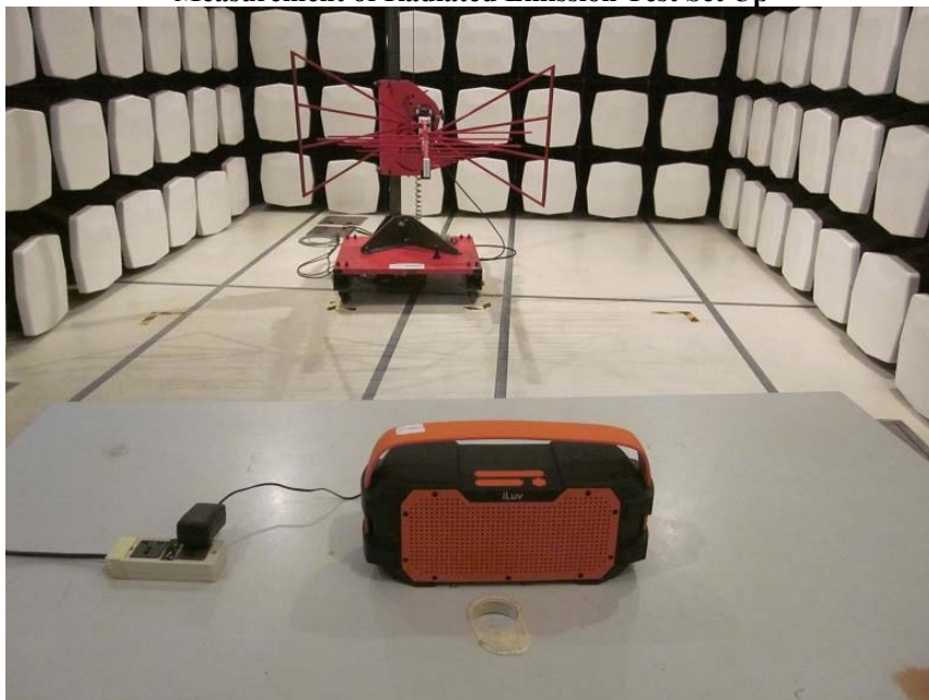
Measurement of Radiated Emission Test Set Up
