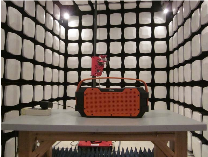
Measurement of Radiated Emission Test Set Up
