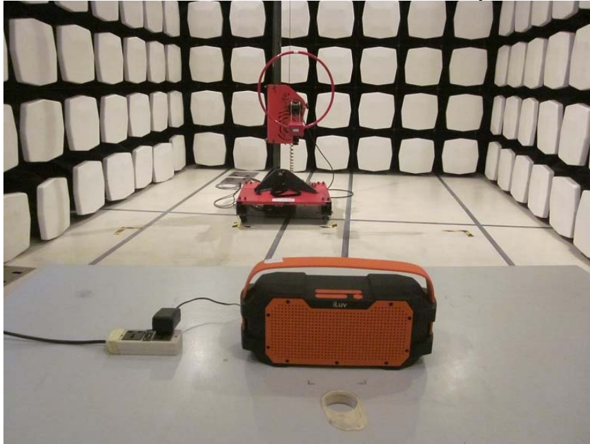
Measurement of Radiated Emission Test Set Up
