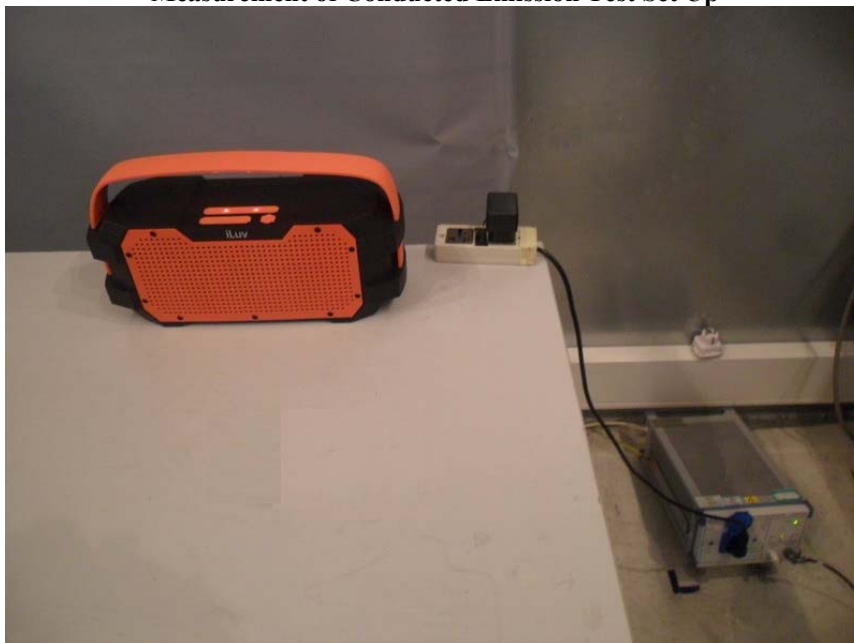
Measurement of Conducted Emission Test Set Up
