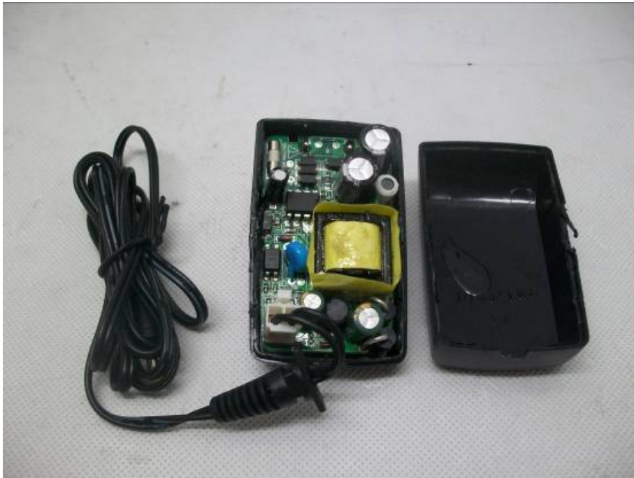
INTERNAL PHOTO OF POWER SUPPLY - 1
