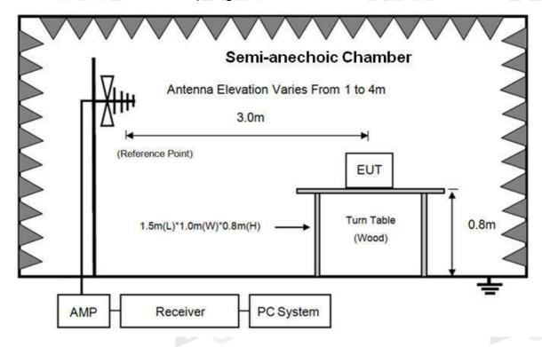
Semi-Anechoic 3m Chamber
