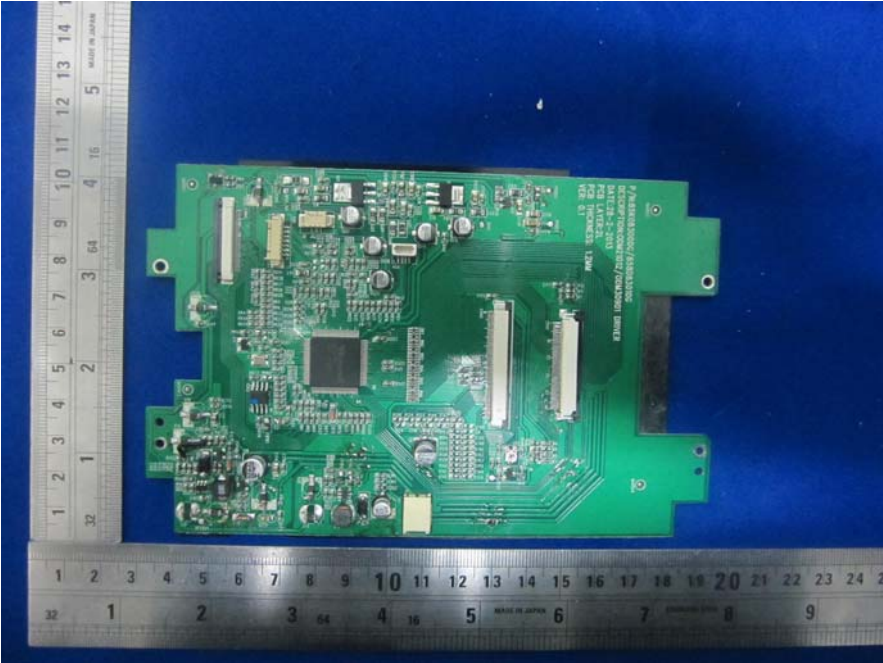
EUT – Screen Board Top view
