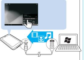
Use the USB cable to connect tablet to PC. You can drag and drop apps and media files between tablet and PC.
