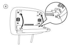
Move the locking tab to right position to fully insert the monitor into the headrest
