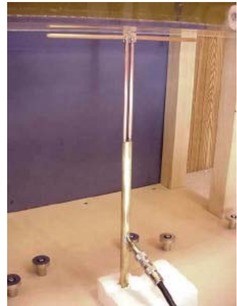
450MHz Dipole Validation Setup
