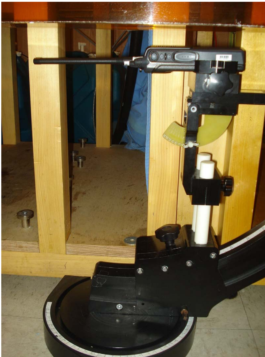
Face-held test setup – Radio with Antenna 1, Battery a
