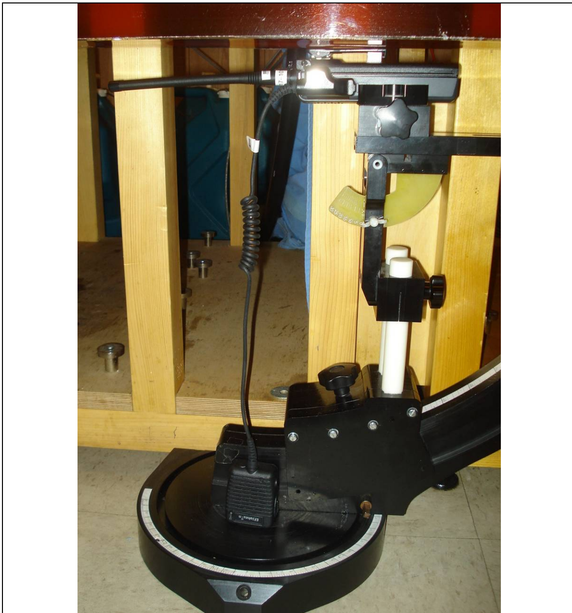
Body-worn Test Setup – Radio with Antenna 1, Body-worn acc. 1, Battery a, Audio acc. 1
