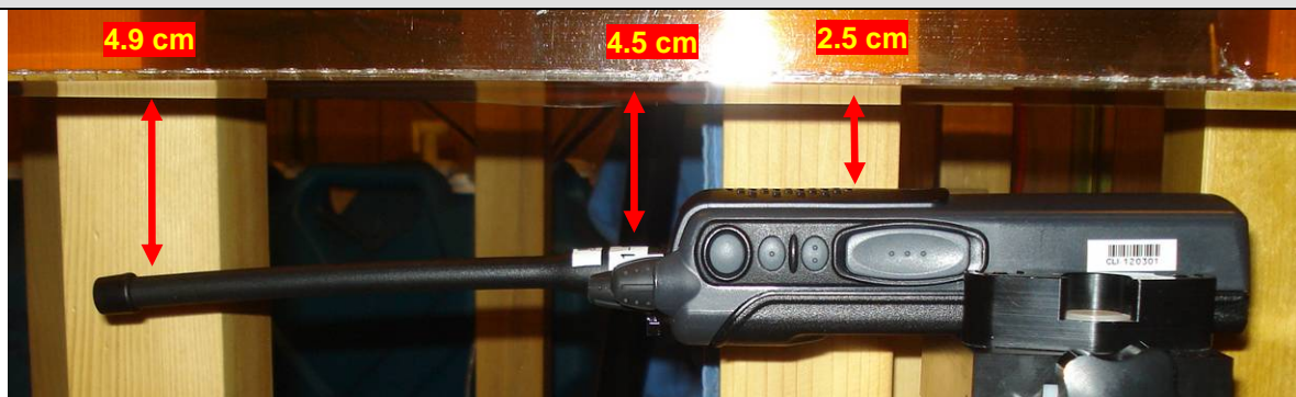
Face-held test setup - Radio with Antenna 4, Battery a
