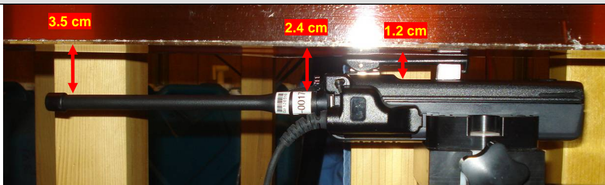
Body-worn Test Setup - Radio with Antenna 4, Body-worn acc. 1, Battery a, Audio acc. 1
