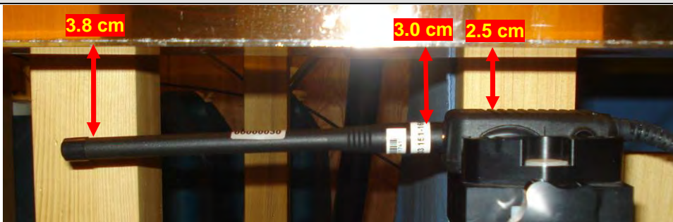
Face-held test setup - Audio acc. 2 with Antenna 2, Battery a
