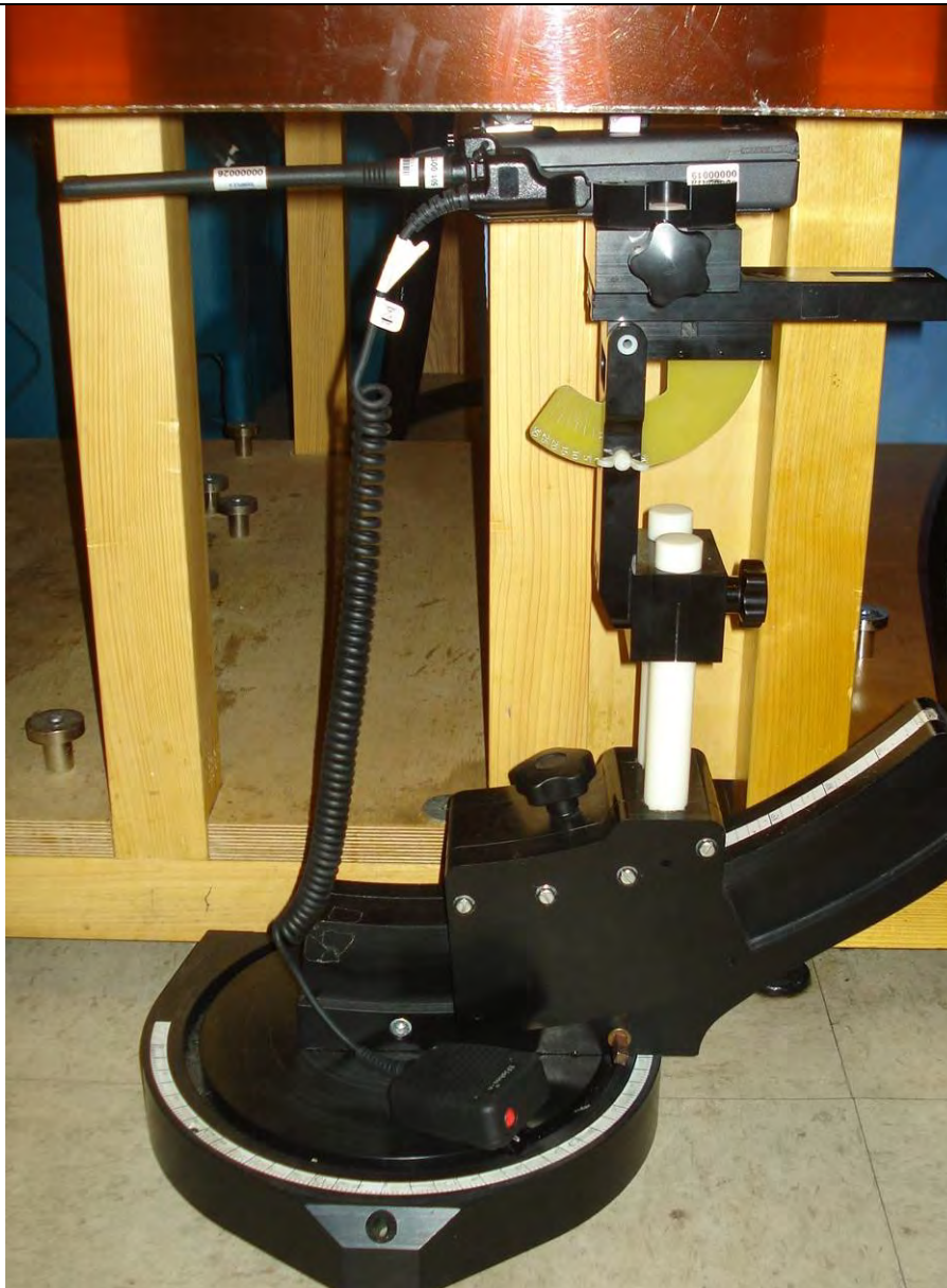
Body-worn Test Setup - VP600 PTT Radio Transceiver
