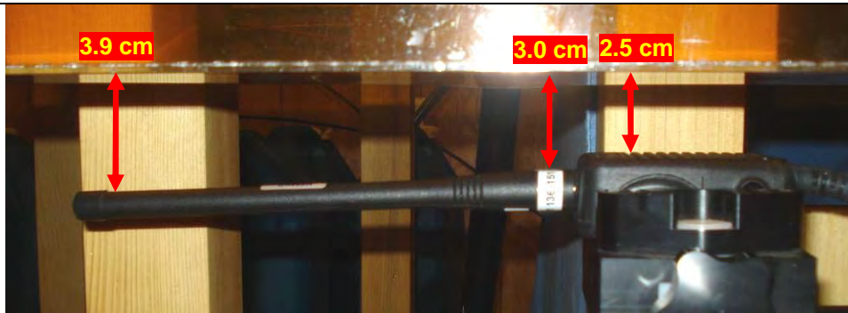
Face-held test setup – Audio acc. 2 with Antenna 1, Battery a
