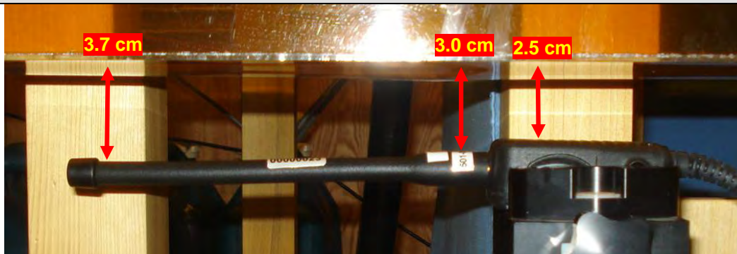
Face-held test setup - Audio acc. 2 with Antenna 4, Battery a
