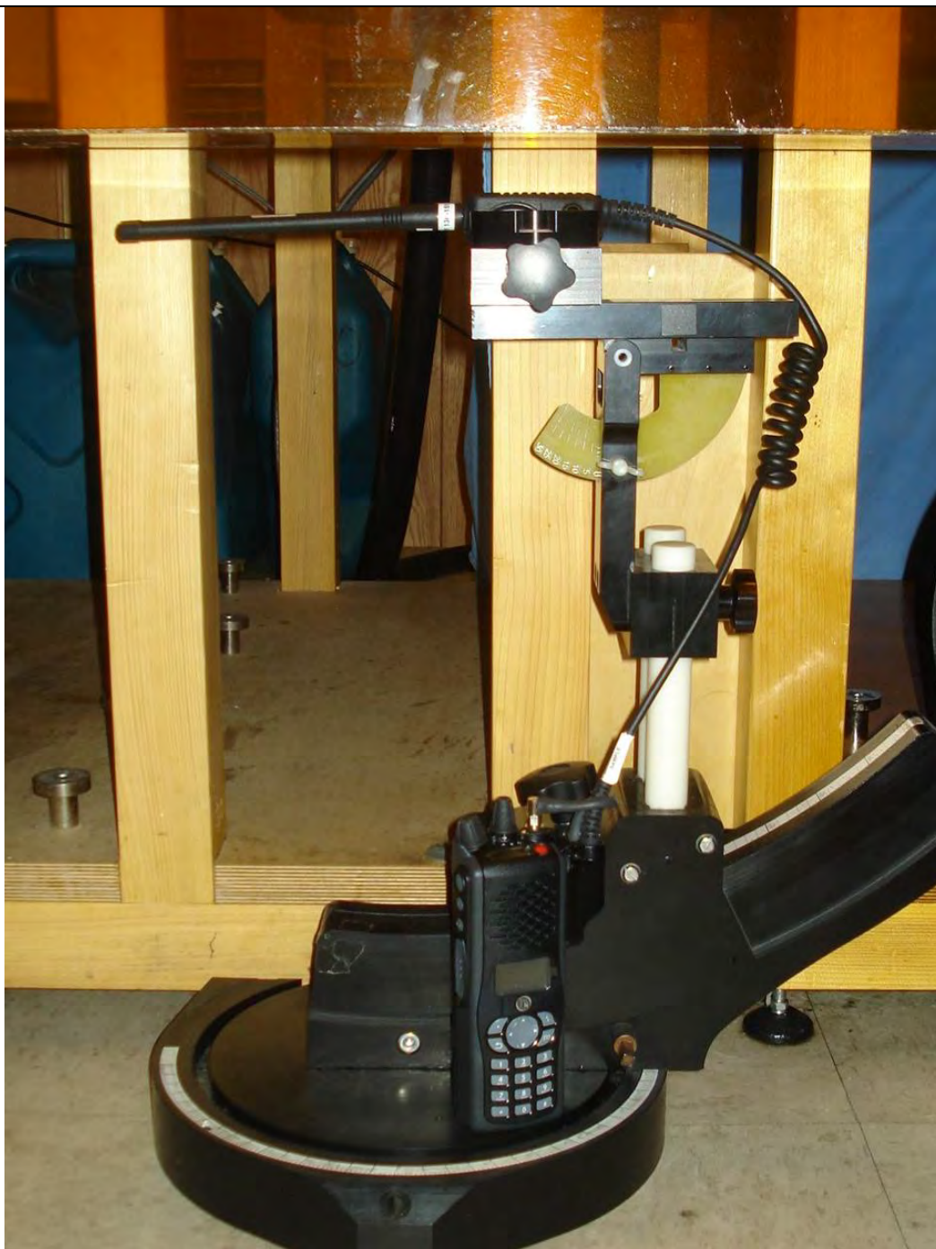
Face-held Test Setup - Speaker-Mic-Antenna accessory connected to VP600 PTT Radio Transceiver
