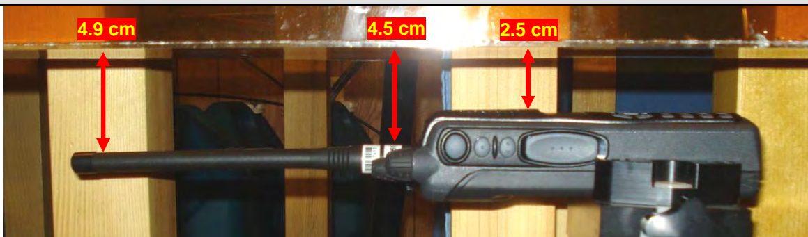
Face-held test setup - Radio with Antenna 2, Battery a
