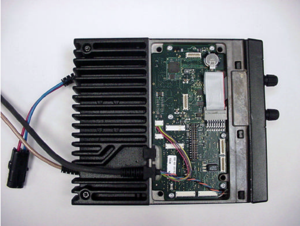
Radio bottom with cover removed showing logic board
