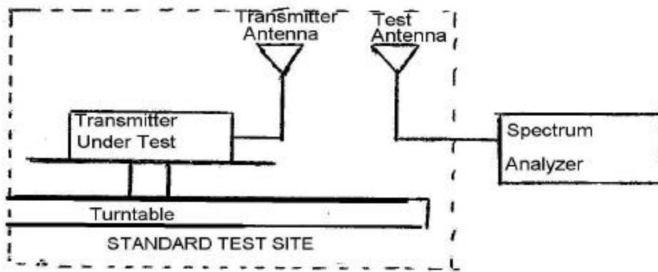
B) Raise and lower the test antenna from 1m to 6 m with the transmitter facing the antenna and record the highest received signal in dB as LVL.
