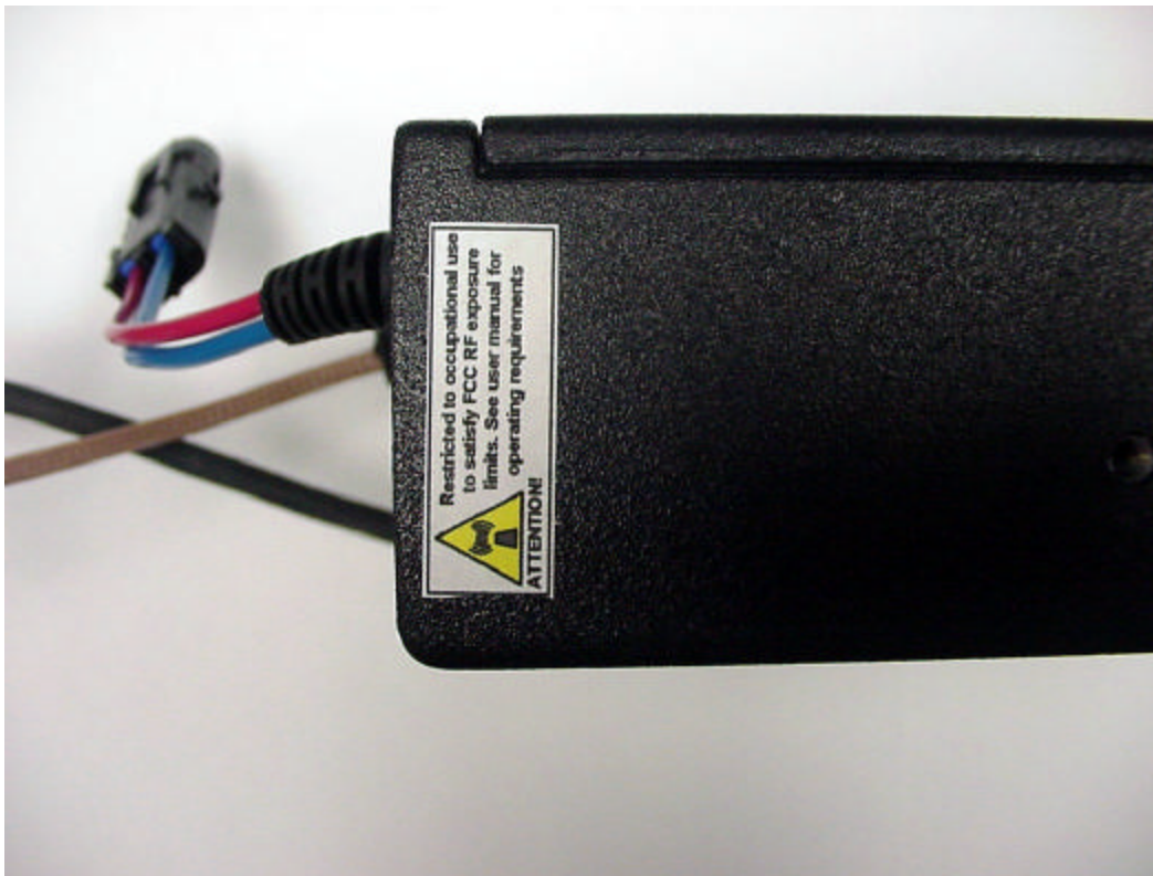
Radio side showing RF safety label
