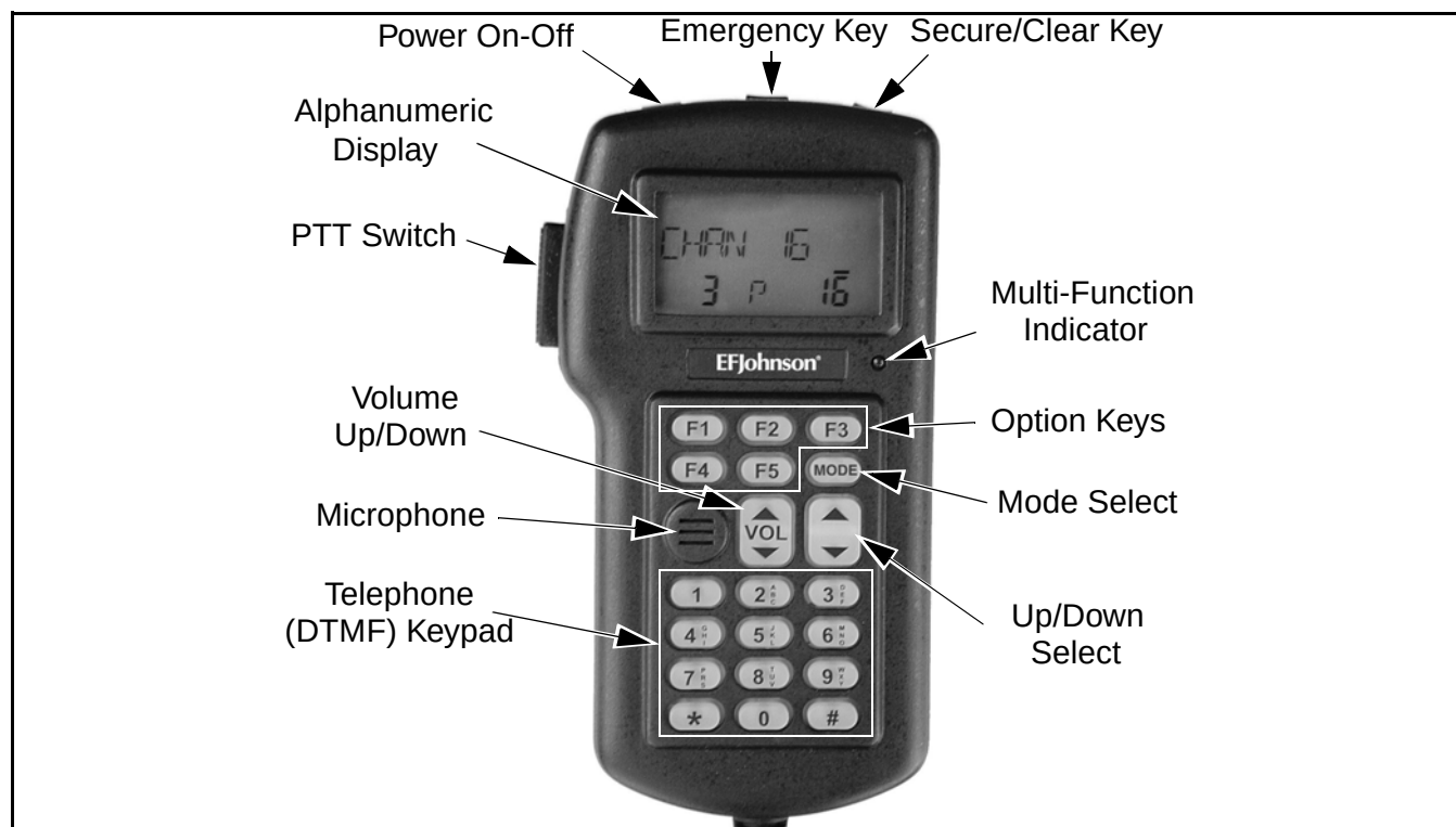
Figure 3-5 Handheld Control Unit Controls
