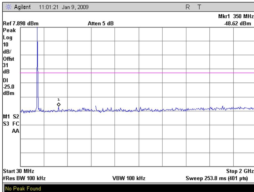
**Name of Test:** Field Strength of Spurious Radiation
