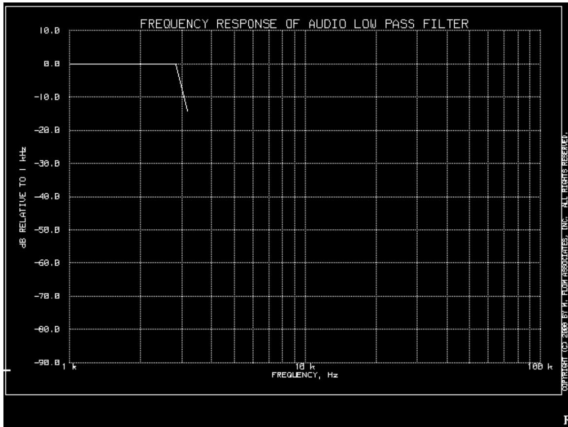
This unit is a digital radio and the roll-off for the filter is very linear in the operational band and sharp out of the band,
