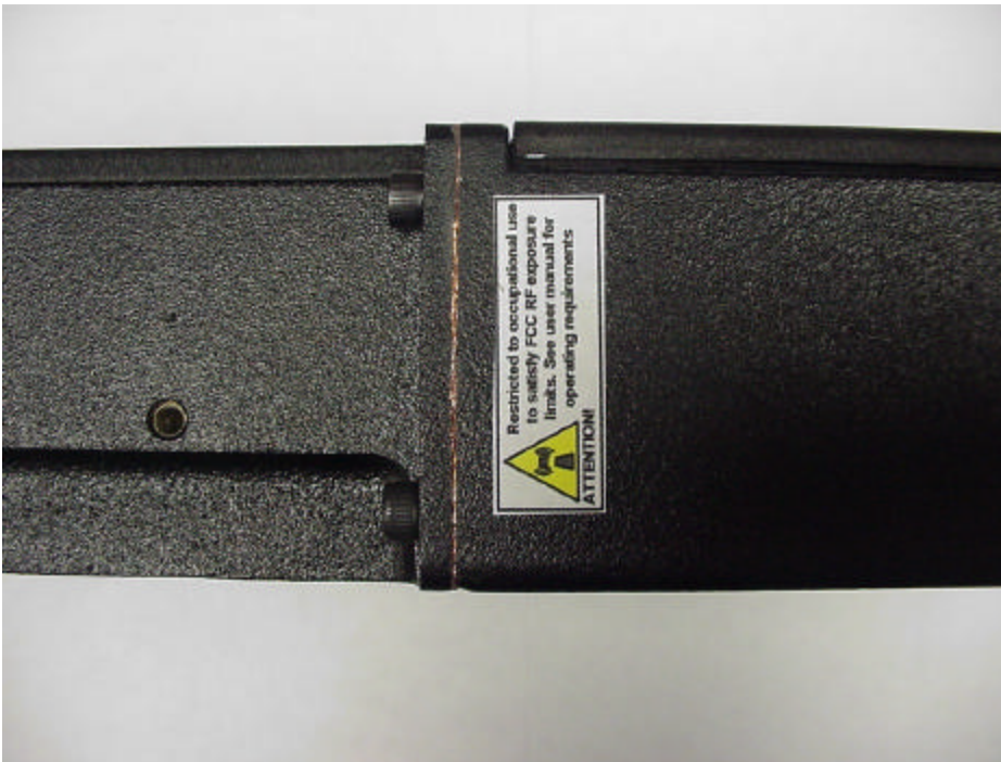
Radio side showing RF safety label
